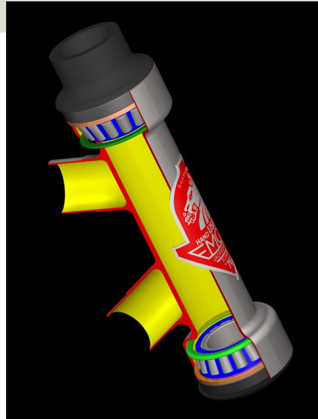
*Using transparency to show the inner workings of the headtube bearing assembly.*
